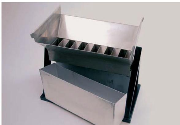
**Fig. 1** Example of a riffle sampler.
