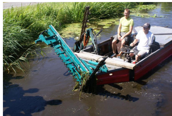
Fig. A2 A weed cutting boat with adjustable mowing gear used to manage invasive alien aquatic plants in the Netherlands © R. Pot.
