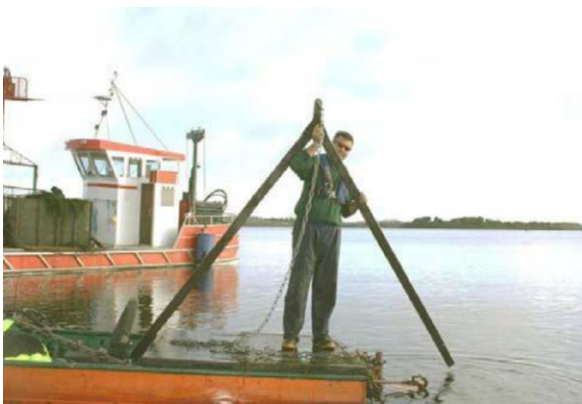
Fig. A1 V-blade used to cut Lagarosiphon major in Rineroon Bay, Ireland (Caffrey & Acavedo, 2007). © Photo reproduced with permission of J. Caffrey, Inland Fisheries Ireland.
