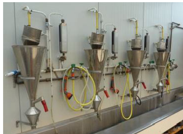
Fig. 9 Oostenbrink elutriator made of stainless steel at Wageningen University, the Netherlands.
