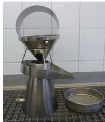
Fig. 14 Left: Vertical-section diagram of Fenwick can. Right: Fenwick can made of stainless steel with 1 mm aperture top sieve displayed in upright position for better visualization (Photo: JKI, Germany).
