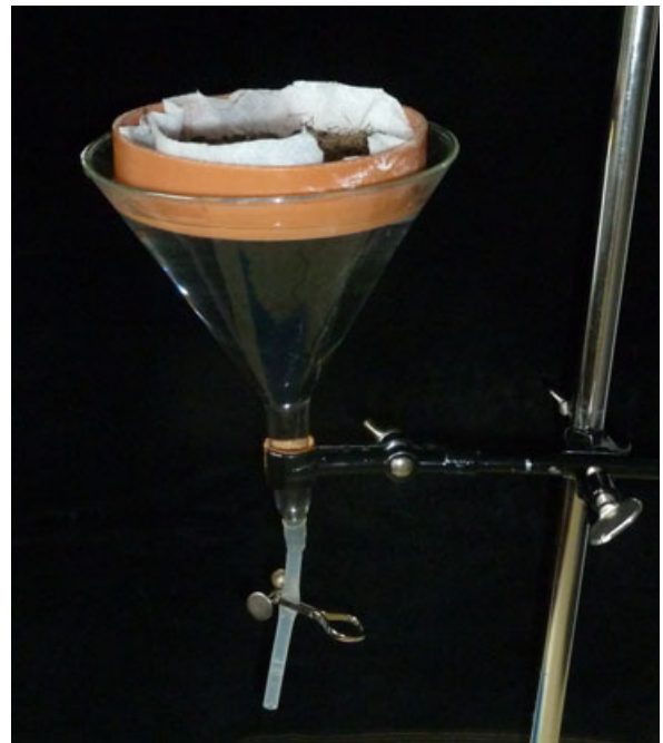
Fig. 1 Modified Baermann funnel for extracting nematodes from plant material or soil (Photo: JKI, Germany).
