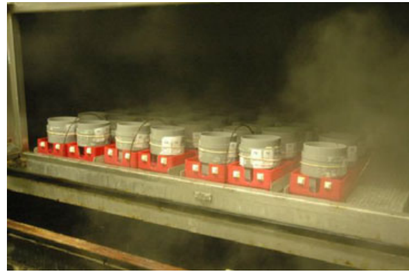
Fig. 5 Mistifier spray apparatus with Oostenbrink dishes used at PPO Lelystad, the Netherlands, with continuous fog (Photo: JKI, Germany).
