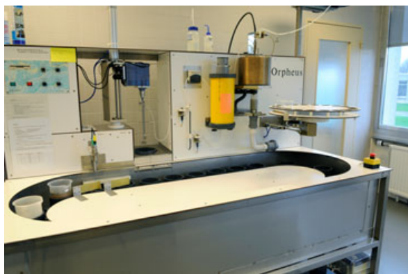
Fig 12 Automated zonal centrifugation. The lower carousel feeds the samples to the centrifuge (1 L beaker) and the upper carousel receives the nematode suspensions (150-mL beaker). The bowl of the zonal centrifuge is kept inside a copper cage for safety reasons. The sample, kaolin and MgSO_4 are fed to the centrifuge bowl through tubes (ILVO, Merelbeke, Belgium).
