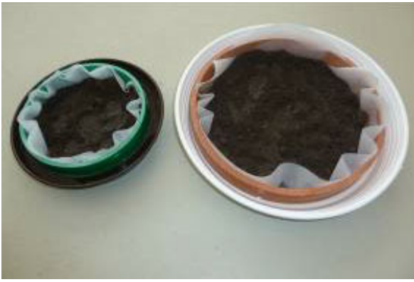
Fig. 6 Oostenbrink dishes for extracting nematodes from soil. Left: Oostenbrink dish with 15 cm inner diameter for samples up to 100 mL soil. Right: Oostenbrink dish with 24 cm inner diameter for samples up to 250 mL soil (Photo: JKI, Germany).
