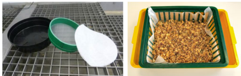
Fig. 2 Oostenbrink dish. Left: Set-up showing plastic dish, supporting sieve made of 250 µm polyamide gauze and cotton-wool milk filter (Photo: JKI, Germany). Right: Set-up consisting of plastic dish, plastic basket and cotton-wool milk filter for extracting Bursaphelenchus xylophilus from wood chips (Photo: Vladimír Gaar, Diag. Lab. Prague, Czech Rep.).
