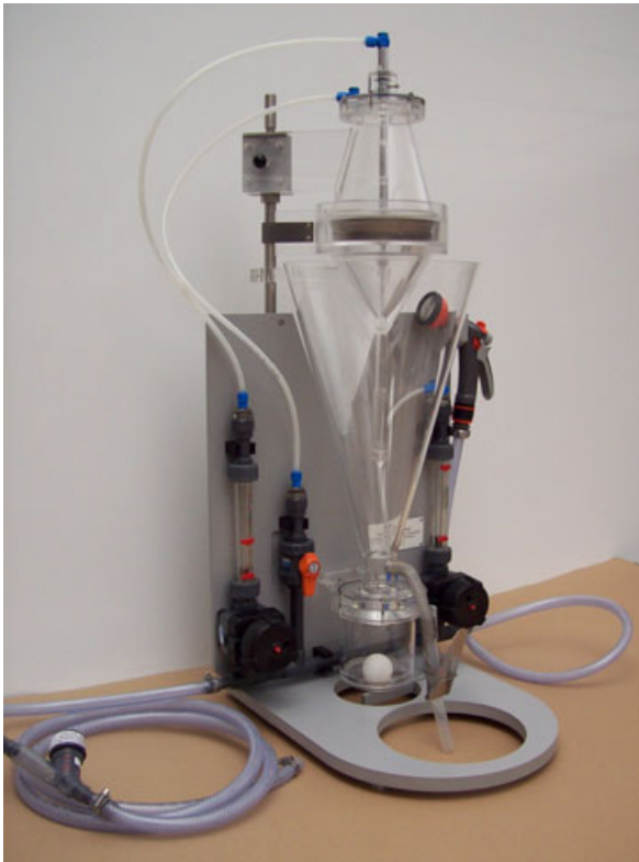
Fig. 10 Modified Oostenbrink elutriator made of acrylic glass (Photo: MEKU, Germany).
