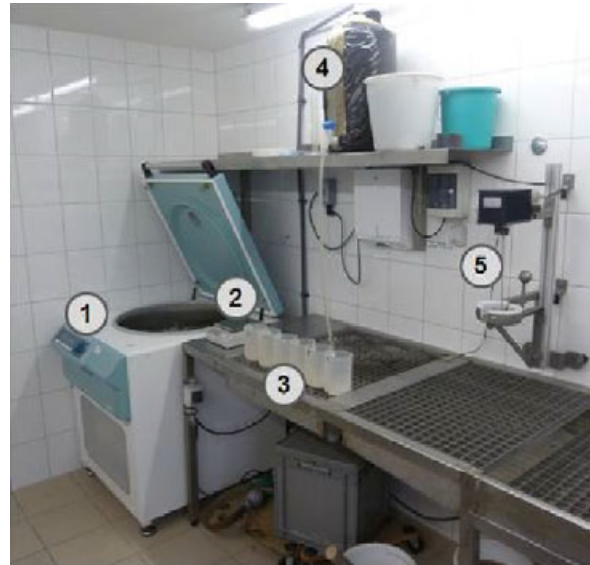
Fig. 11 Equipment used for centrifugal flotation; (1) centrifuge, (2) balance (scale), (3) centrifuge tubes, (4) container with \text{MgSO}_4 solution, (5) Vibro mixer (JKI, Münster, Germany).
