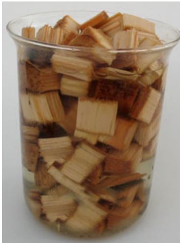
Fig. 3 Extraction of a chopped wood sample in a glass beaker (Photo: Tomasz Konefał, Toruń, Poland).
