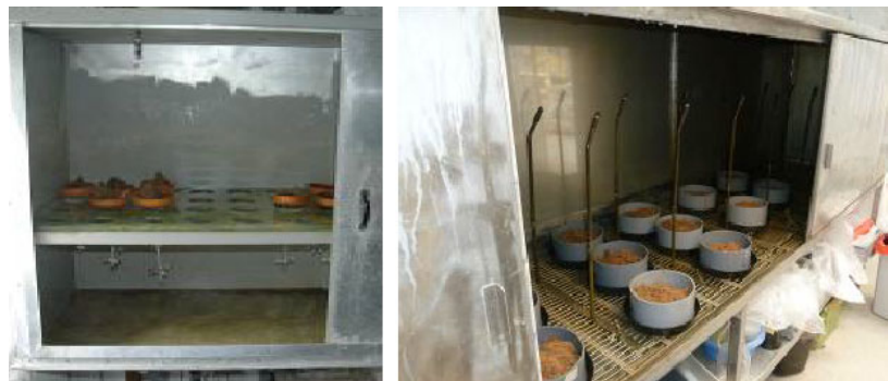
Fig. 4 Left: Mistifier spray apparatus with Baermann funnels used at the Julius Kühn-Institute in Münster, Germany, with water spraying from the top directly onto the samples. Right: Mistifier spray apparatus with Oostenbrink trays used at Wageningen University, the Netherlands, with water spraying from the bottom to the top and then falling onto the sample (Photos: JKI, Germany).
