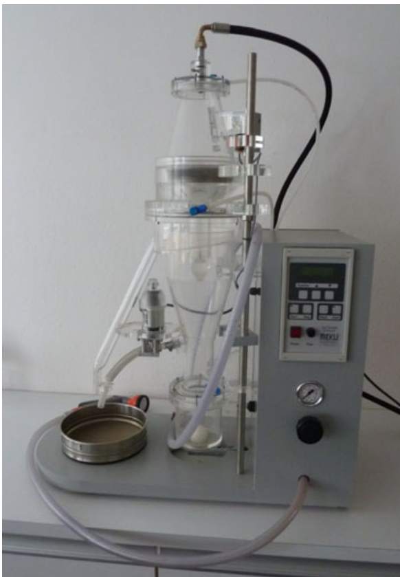
Fig. 20 Automated soil sample extractor for cysts (Photo: JKI, Germany).
